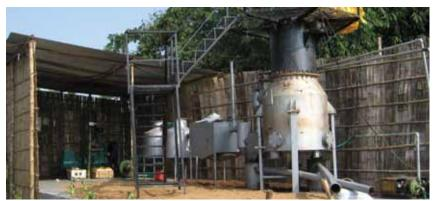
Husk Power Systems has pioneered a new way of providing electricity to rural India through the gasification of rice husk.
